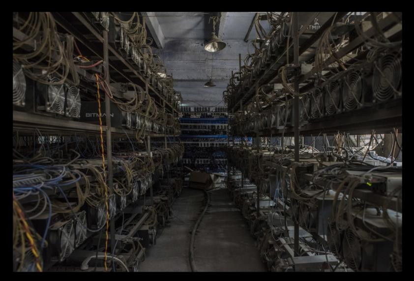
Racks of mining machines line the shelves at a server farm in Guizhou. The computers try to unlock new Bitcoins by solving computational problems and serving as accountants for the Bitcoin network. The machines are used to mine Bitcoin and Ether, a competing virtual currency.
